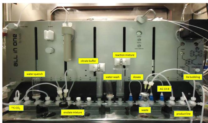
Fig. 2. TRASIS AIO reaction setup for  $[^{11}\text{C}]\text{AcAc}$  radiosynthesis.
